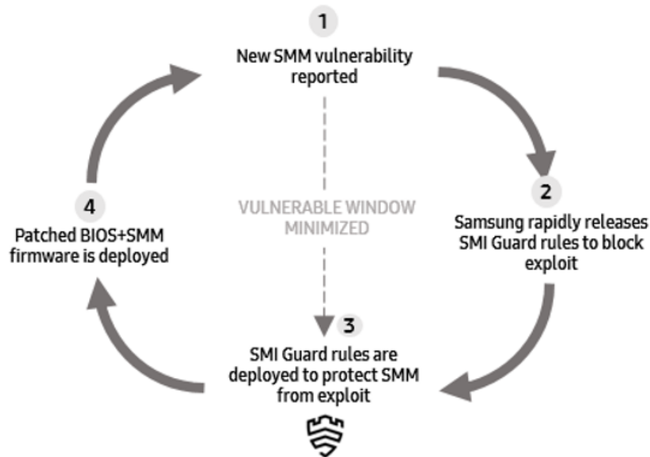
Figure 4: SMI Guard enables rapid incident response and minimizes the window of vulnerability
